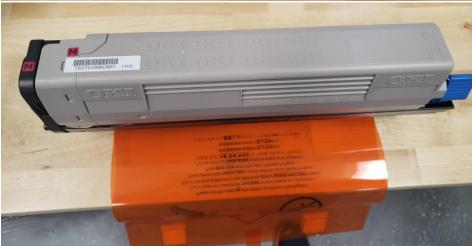
a. Make sure that you lock the toner to the drum assembly before picking them back up and putting back in the printer
